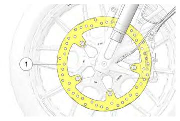
Clean discs if minor squeaks develop due to dirt or dust. Apply brake cleaner to a clean shop towel and wipe the discs. DO NOT allow brake cleaner to contact painted or plastic parts. Read all precautions on the label.
