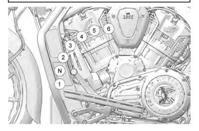
This motorcycle is equipped with a six-speed transmission. Neutral is located between first and second gear.
