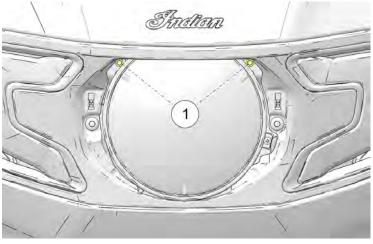
The headlamp adjustment screws ① are located inside the headlamp housing.
