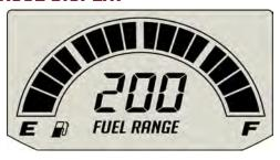
The fuel gauge displays fuel level. For the most accurate reading, sit on the motorcycle and bring it to the upright position.
