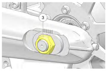
6. Turn the RIGHT SIDE adjuster nut ④ to achieve proper belt tension
