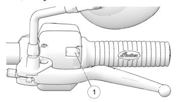
The power switch must be ON for the toggle switches to function. Use the right-hand switch to navigate through menus or accept dialog boxes on the Ride Command display. Use the left-hand switch to back out of menus, decline dialog boxes, hang up phone calls, and toggle through display screens.
