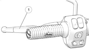
Freeplay (gap) is the amount of lever movement from the rest position to the point of cable resistance. Clutch lever freeplay should be 0.5-1.5 mm. Measure the gap between the clutch lever and the lever housing. See page 116. Adjust clutch lever freeplay if necessary.
