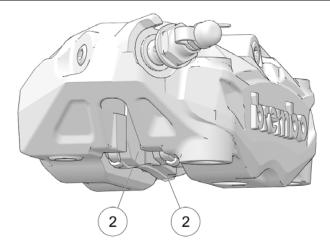
Inspect each front brake pad on both sides of the front disc. Inspect each rear brake pad on both sides of the rear disc. Replace brake pads when the thinnest point of the friction material ② has worn to 1.0 mm. Please see your dealer for this service.
