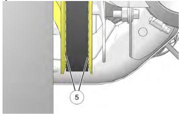
If necessary, loosen the axle nut and LEFT SIDE adjuster until belt just moves off the right flange and begins to track down the center of the driven sprocket flange during forward wheel rotation.
