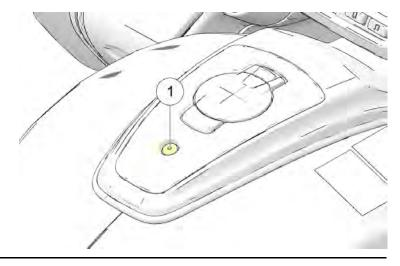
1. Ensure engine is not running before attempting to manually unlock fuel cap
