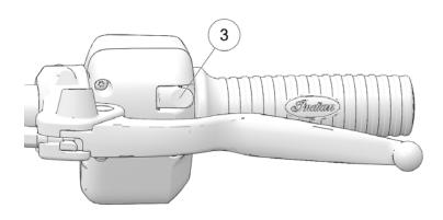
There are trigger switches located on the reverse side of both the right and left  $\Im$  switch cubes.
