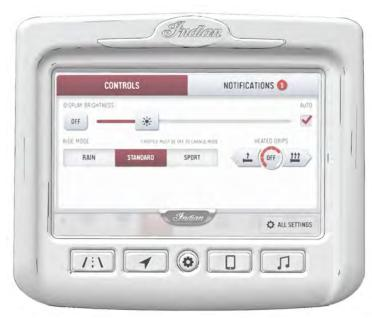
From the Control Panel you can access settings, adjust display brightness, select ride mode, and vehicle climate controls.
