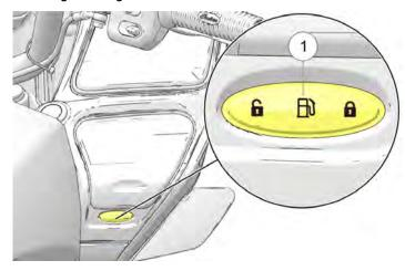
2. Press the full cap release button  $\ensuremath{\textcircled{2}}$  to access the fuel tank.
