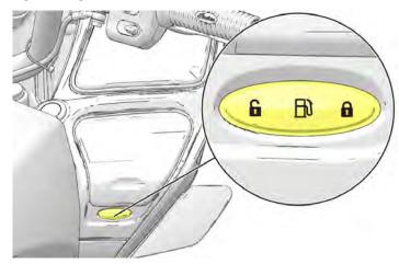
Press the fuel cap release button ① (previous page) to release spring loaded cap.
