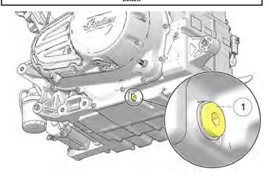
4. Remove the drain plug. Allow the oil to drain completely.
