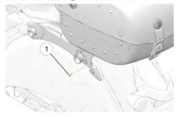
2. Lift the trunk latches (2) to unlock the trunk from the mount.
