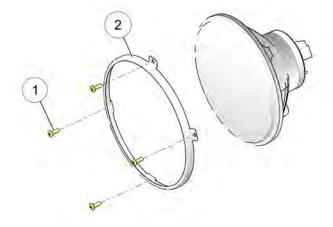
3. Remove the headlight assembly from the headlight carrier.
