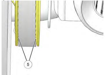
If necessary, loosen the axle nut and LEFT SIDE adjuster until belt just moves off the right flange and begins to track down the center of the driven sprocket flange during forward wheel rotation.
