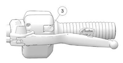
There are trigger switches located on the reverse side of both the right and left  $\ensuremath{\Im}$  switch cubes.
