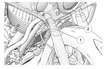
Clean the fork tubes to remove bugs, tar or buildup which may cause seal wear or leakage. Inspect the outer surfaces of the inner fork tubes for scratches or damage from foreign objects.
