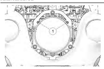
Remove the two headlight bezel screws (fairing models only)
