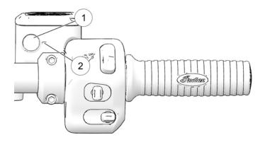
5. Reinstall the diaphragm, cover and screws.
