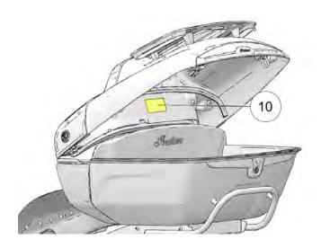
10 Trunk/Trunk Rack Capacity Label
