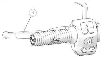
Freeplay (gap) is the amount of lever movement from the rest position to the point of cable resistance. Clutch lever freeplay should be 0.5-1.5 mm. Measure the gap between the clutch lever and the lever housing. See page 122. Adjust clutch lever freeplay if necessary.
