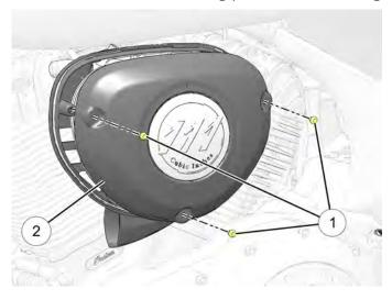
2. Remove the three air filter screws ③ and remove the air filter assembly.
