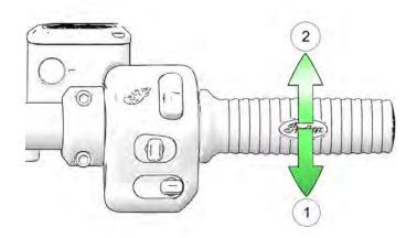
The control grip is spring loaded. When you release the grip, the throttle returns to the idle position.
