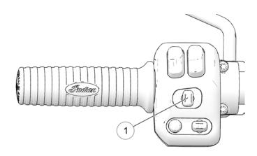
To activate the hazard switch, press on the center of the turn signal switch 1.
