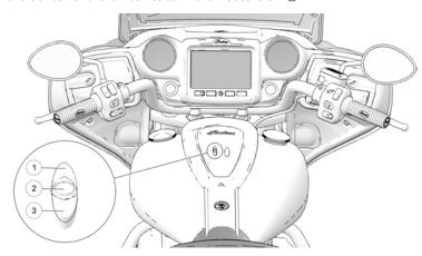
The heaters have 10 heat levels, ranging from OFF (level 0) to highest heat (level 10). Press and release the top of the switch 1 to increase the heat level by one increment. Press and release the bottom of the switch 3 to decrease heat by one increment.
