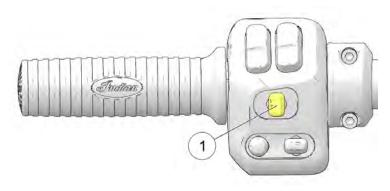
To activate the hazard switch, press on the center of the turn signal switch (1).
