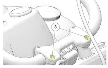
8. Rotate the handlebar into the desired position and torque the riser clamp fasteners to specification.
