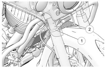
Clean the fork tubes to remove bugs, tar or buildup which may cause seal wear or leakage. Inspect the outer surfaces of the inner fork tubes for scratches or damage from foreign objects.
