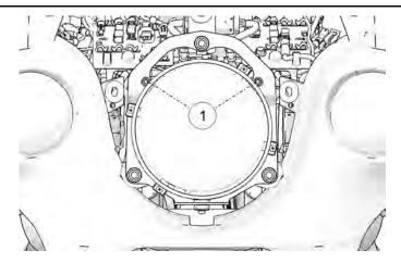
1. Remove the two headlight bezel screws (*fairing models only*) and remove the bezel from the fairing. Reinstall the bezel after adjusting the headlamp.
