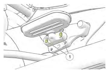
To adjust the height, remove both attachment screws. Move the floorboard assembly to the next hole position, then reinstall the fasteners, adjust the angle and tighten the fasteners.
