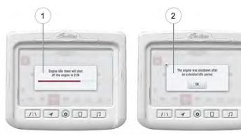
For motorcycles equipped with Ride Command, a notification will display a countdown timer to warn that the engine is about to shut off (1). After the time has elapsed and the engine is shut off, a subsequent notification will be displayed (2). After the engine shuts off, the engine can re-started by pressing the starter switch.
