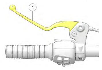
2. Freeplay (gap) is the amount of lever movement from the rest position to the point of cable resistance. Clutch lever freeplay should be 0.5-1.5 mm. Measure the gap between the clutch lever and the lever housing. See page 120. Adjust clutch lever freeplay if necessary.
