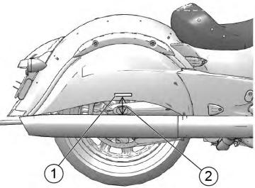
Periodically inspect rear shock preload. For the most comfortable ride and proper ground clearance, adjust preload if ride height is out of specification.
