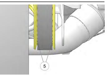
3. If necessary, loosen the axle nut and LEFT SIDE adjuster until belt just moves off the right flange and begins to track down the center of the driven sprocket flange during forward wheel rotation.
