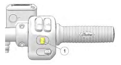
Cruise control can be activated and adjusted from the right control using the Cruise Control Switch (1).
