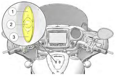
The heaters have 10 heat levels, ranging from OFF (level 0) to highest heat (level 10). Press and release the top of the switch (1) to increase the heat level by one increment. Press and release the bottom of the switch (3) to decrease heat by one increment.
