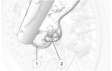
2. Inspect for debris adhering to the end of the wheel speed sensors (2). If contamination is observed, or if you are unable to visually inspect, slide a thin towel across the face of the sensor between the sensor and the tone ring to remove any potential debris.
