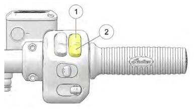
Press the top of the switch (STOP) 1 to interrupt the circuits and stop the engine. The engine should not start or run when the switch is in the STOP position.
