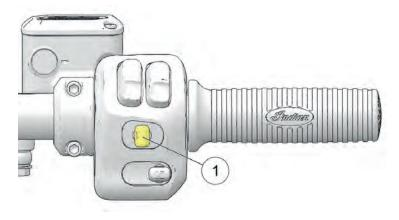
Cruise control can be activated and adjusted from the right control using the Cruise Control Switch (1).
