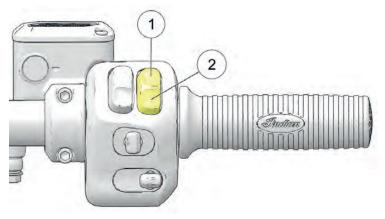
Press the top of the switch (STOP) (1) to interrupt the circuits and stop the engine. The engine should not start or run when the switch is in the STOP position.
