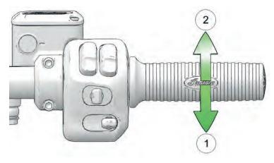
The control grip is spring loaded. When you release the grip, the throttle returns to the idle position.
