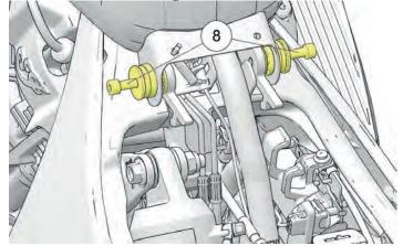
13. Lift rear of tank upward and pull rearward to remove. Place the fuel tank in a secure location with a drain pan to catch any fuel than may leak or drip from disconnected hoses or fittings.
