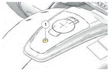
2. With fastener removed, lift the rear of console enough to clear fuel cap and push forward to release front mount from keyway.
