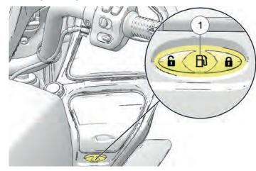
2. Press the full cap release button (2) to access the fuel tank.
