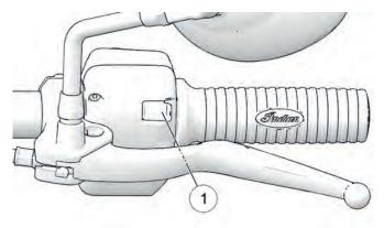
The power switch must be ON for the toggle switches to function. Use the right-hand switch to navigate through menus or accept dialog boxes on the Ride Command display. Use the left-hand switch to back out of menus, decline dialog boxes, hang up phone calls, and toggle through display screens.
