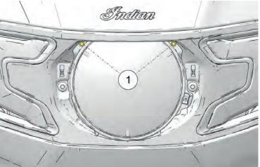
The headlamp adjustment screws () are located inside the headlamp housing.
