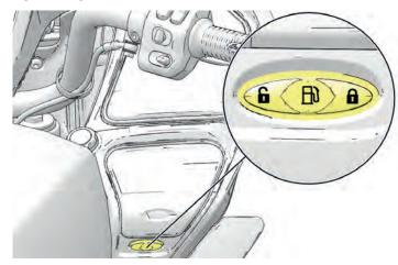
2. Press the fuel cap release button (2) (previous page) to release spring loaded cap.
