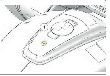
1. Ensure engine is not running before attempting to manually unlock fuel cap
