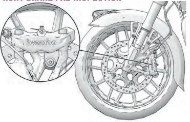
Inspect each front brake pad on both sides of the front discs. Inspect each rear brake pad on both sides of the rear disc. Replace brake pads when the thinnest point of the friction material (2) has worn to 1.0 mm. Please see your dealer for this service.
