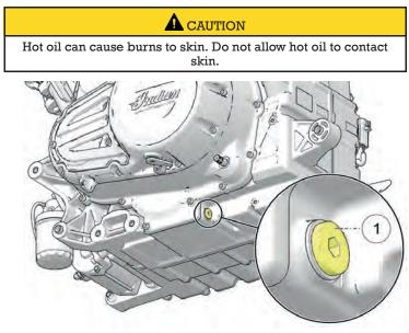
4. Remove the drain plug. Allow the oil to drain completely.
