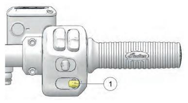
Press up on the switch to adjust the windshield upward. Press down on the switch to adjust the windshield downward. Double tap up or down on the switch to auto-adjust the windshield all the way up or down. If the windshield is traveling and the opposite direction is briefly pressed, the auto travel is canceled.
