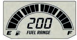
For the most accurate reading, sit on the motorcycle and bring it to the upright position before turning it on.
