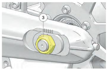
6. Turn the RIGHT SIDE adjuster nut (4) to achieve proper belt tension
