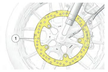
2. Clean discs if minor squeaks develop due to dirt or dust. Apply brake cleaner to a clean shop towel and wipe the discs. DO NOT allow brake cleaner to contact painted or plastic parts. Read all precautions on the label.
